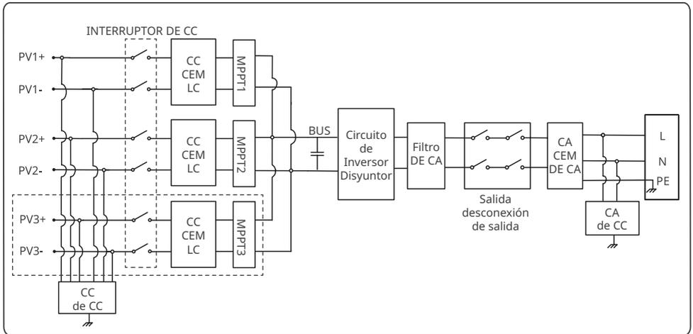
PV3+/PV3- solo para GW5000-MS-30, GW6000-MS-30, GW7000-MS-30, GW8500-MS-30, GW9900-MS-30, GW10K-MS-30.
