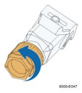
step 2 Thread the AC cable of appropriate length through the swivel nut, the sealing ring and the housing.
