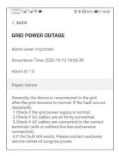
figure 7-9 Detailed Fault Alarm Information
