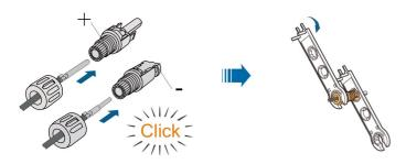
step 4 Check for polarity correctness.
