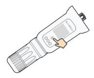
figure 7-1 Enabling the WLAN Hotspot
