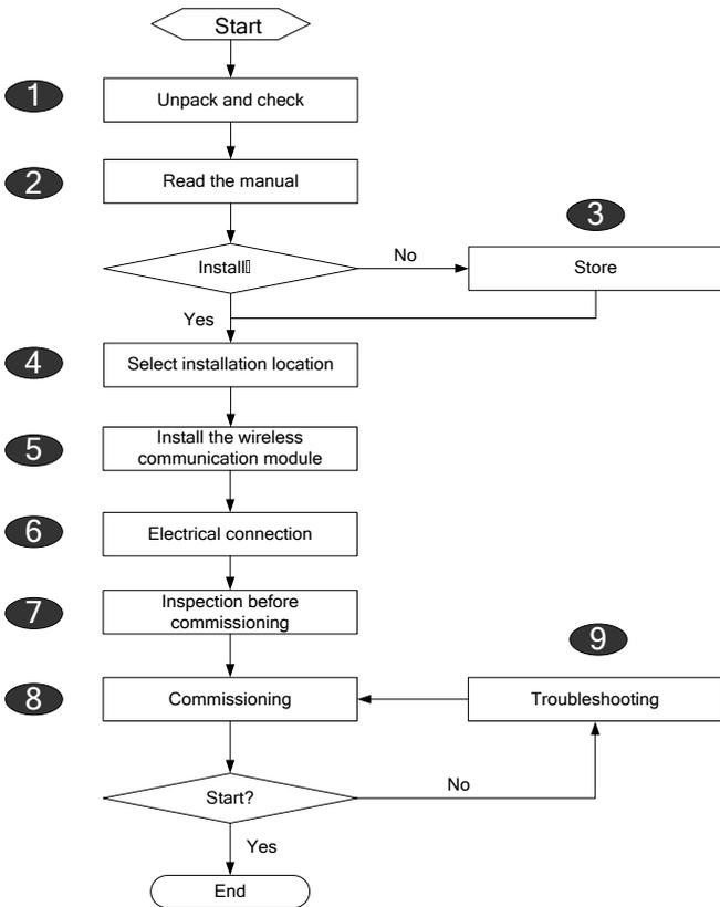
Fig. 3-1 Installation Flow
