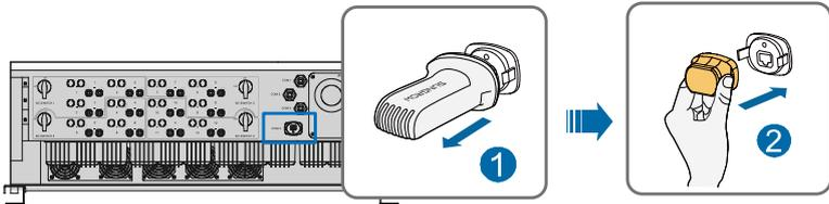
**Step 2** Pack the wireless communication module in its original packing case and seal the RJ45 interface at the bottom of the inverter with supplied waterproof plug.
