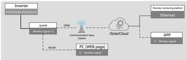
**Fig. 2-3** Application of the wireless communication module (4G+WLAN)
