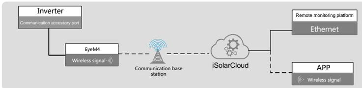
**Fig. 2-2** Application of the wireless communication module (4G)
