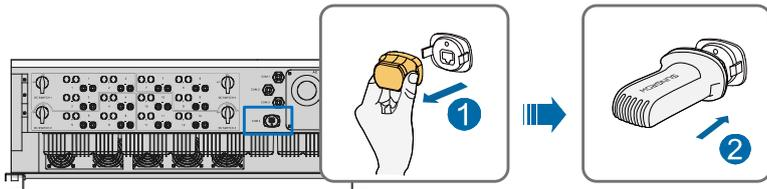
**Step 2** Insert the wireless communication module into the network port (COM) at the bottom of the inverter until it snaps into place with a "Click" sound. If the module is still loose, remove it from the communication port and check whether the port is damaged. If the port is normal, reinsert the wireless communication module.
