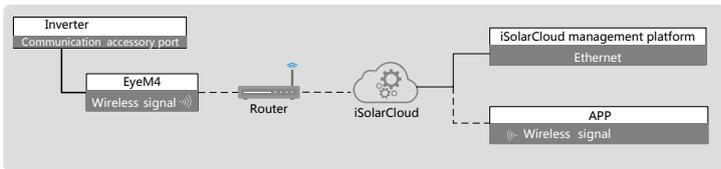
**Fig. 2-1** Application of the wireless communication module (WLAN)
